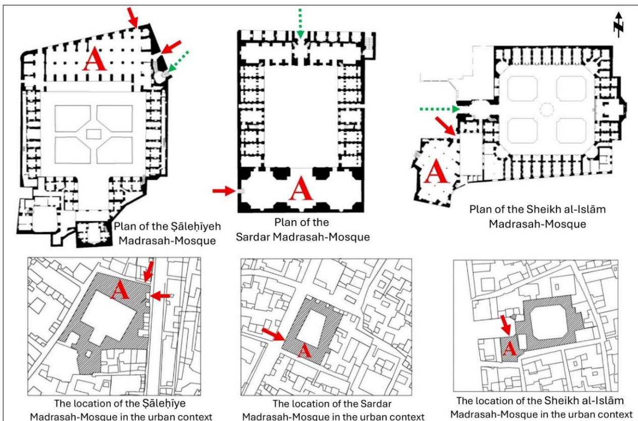
A Figure 11. Location of the Prayer Space (Prayer Hall–Mosque) in the Sheikh al-Islam, Sardar, and Salehieh Madrasa-Mosques (Plan Sources: Qazvin Province Cultural Heritage Documentation Center, 2010 , Document Nos. 102–104). Red arrow: Direct access from the urban fabric to the prayer spaces (prayer hall–mosque) allows public use, while the Green dashed arrow: the main entrance (iwan) serves the residents of the madrasa (students, instructors, etc.) in accordance with traditional Iranian architectural patterns, maintaining spatial hierarchy. In the historical Madrasa-Mosques of Qazvin (excluding Peyghambariyeh), a separate direct access
